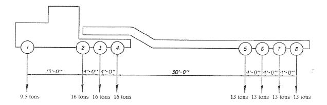
Maximum Allowable Special Vehicle 2 Loading: Maximum Allowable Axle Load for Special Vehicle 2
