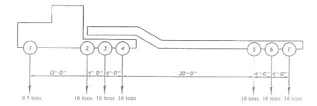
Maximum Allowable Special Vehicle 3 Loading: Maximum Allowable Axle Load for Special Vehicle 3
