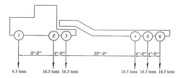
Maximum Allowable Special Vehicle 4 Loading: Maximum Allowable Axle Load for Special Vehicle 4
