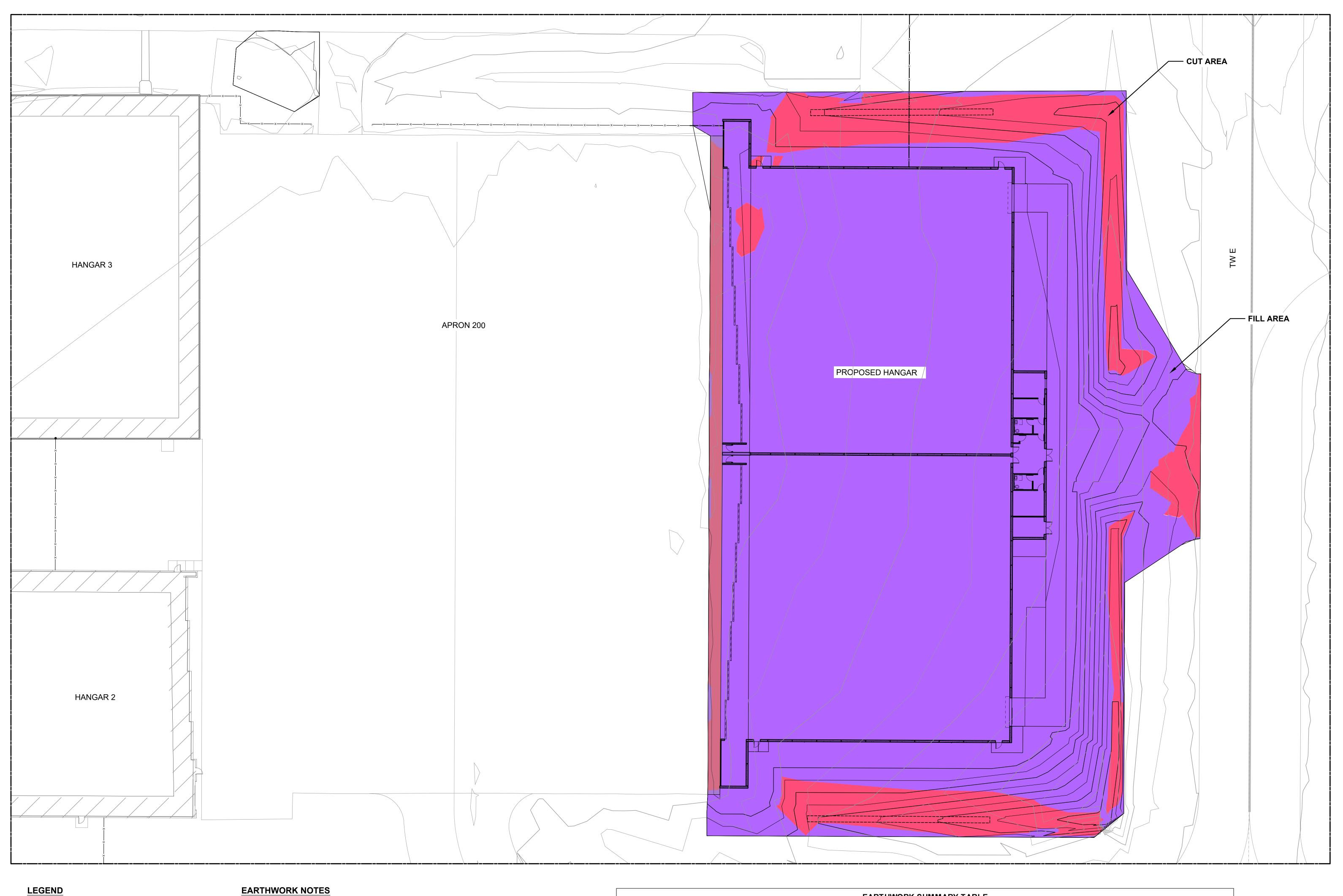
EARTHWORK SUMMARY TABLE 8" TOPSOIL 6" TOPSOIL PLACEMENT EXCESS TOPSOIL CUT FILL STRIPPING AVG. LOCATION **BORROWED EXCAVATION** (CUBIC YARDS) (CUBIC YARDS) (CUBIC YARDS) (CUBIC YARDS) (CUBIC YARDS) (CUBIC YARDS) FILL SITE GRADING 423.9 3636.7 3212.7 1974.7
